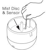
Use a cotton swab with warm water, gently clean the mist disc and sensor located at the inside bottom of the base.
