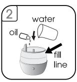
Using a cup, fill with regular tap water up to the max fill line.
