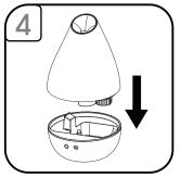
Replace the tank back onto the base.
