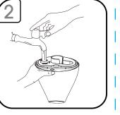
Remove cap and fill to slightly below capacity with luke warm water.
