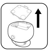
Remove the battery cover from the base.
