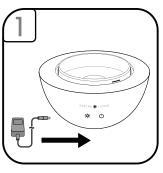
Plug the power to the unit first then connect to wall outlet.
