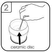
Using a cotton swab with warm water, gently clean the ceramic disc to remove oil residue.
