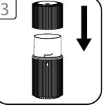
Lower cover onto base. Turn clockwise to secure.
